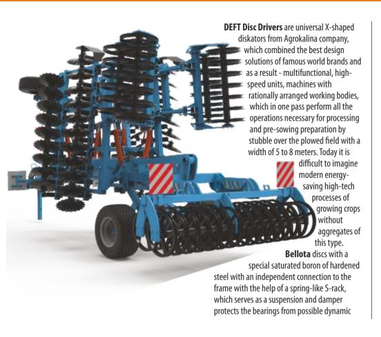
loads. Spring 3D rack - due to the displacement of the disk in three planes, allows you to better copy the field microrelief. **DEFT** units are equipped with maintenance-free double-row radial-thrust bearing units of the closed type FKL, which do not require periodic maintenance and have a 2-year warranty from the manufacturer. The wheel units from **STARCO** provide durable, reliable operation in various climatic and field conditions.
