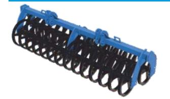
Self-cleaning double steel roller with grinding effect and low adhesion. The rings of the rink are arranged in a checkerboard pattern; during operation, they are self-cleaning from adhering soil. The roller performs the following functions:
