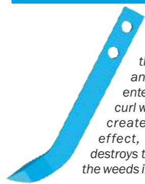
The tooth has the shape of a spike, flattened, pointed at the end and bent at an angle, allows the tooth to enter the soil at 90° and curl when leaving the soil to create a micro-explosion effect, thus it completely destroys the crust and pulls out the weeds in the thread stage.
